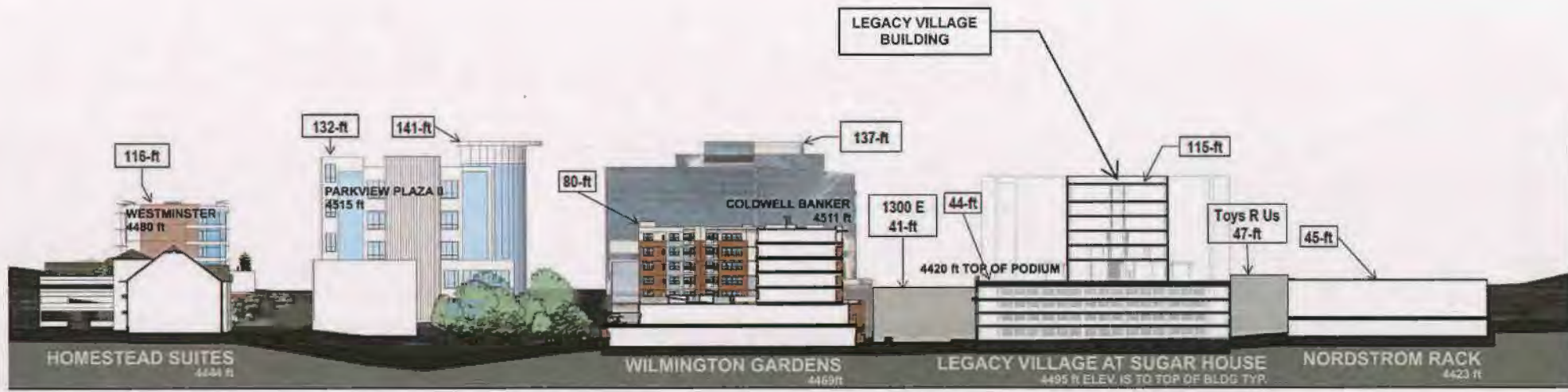
Site Cross-Section Exhibit (Shows relative height of Legacy Village Building to other surrounding buildings)
