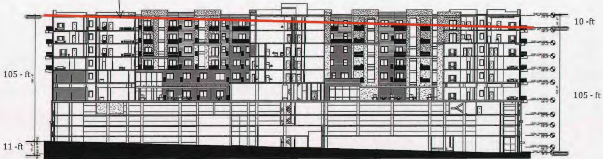
Grade Change Exhibit (Cross-section cut along south side where the greatest change in grade occurs)
